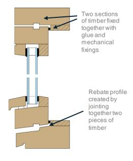
Frame created from separate sections of timber
